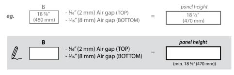
Note: when the top of the DishDrawer<sup>®</sup> has to be lower than the adjacent cabinetry, the panel can be increased in height.
